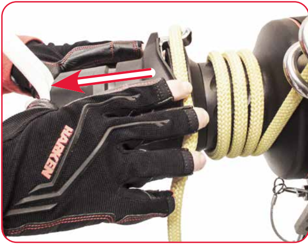
Check the mobility of the semi-pulley cover.
