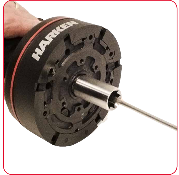
5. Lock the screw on the handle coupling.
