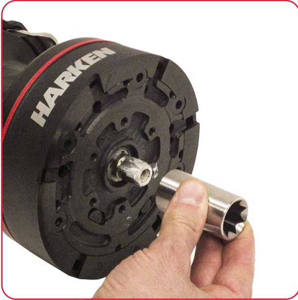
4. Position the handle coupling on the shaft.
