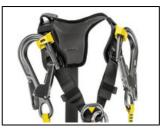
The MGO connectors on fall-arrest lanyards can be stowed on each shoulder strap. The user is thus unhindered by the lanyard, and the connectors stay within reach. In the event of a fall, the system releases the MGOs and allows the absorber to be deployed.
