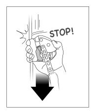
• After locking, verify that the device unlocks normally.
