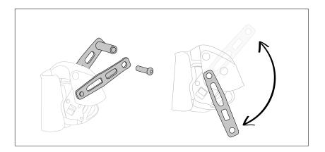
• Install the energy absorber and close the clevis. Use thread-locking fluid on the screw. Check the tightness of the screw.
