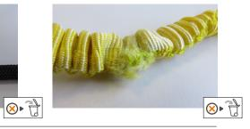
• Worn pouch, absorber is unprotected
