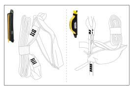
• Check the condition of the safety stitching on both sides. Look for any threads that are loose, worn, or cut.
