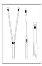
• Check the condition of the safety stitching on both sides. Look for any threads that are loose, worn, or cut.
