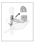
• Open the pouch and pull out the energy absorber.
