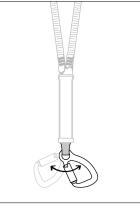
• Or move the connector to inspect the hidden parts.
