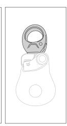
• Check the condition of the attachment holes (marks, deformation, cracks, wear, corrosion...).
