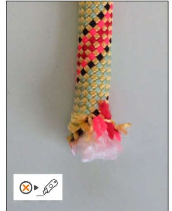
• Damaged rope end
