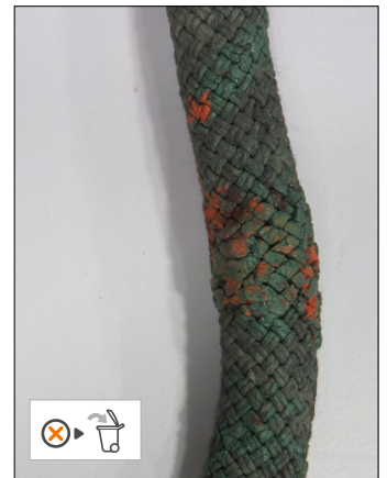
• Trace of paint
