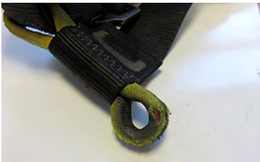
• Damaged attachment point
