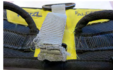
• Damaged attachment point
