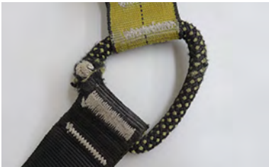
• Damaged attachment point
