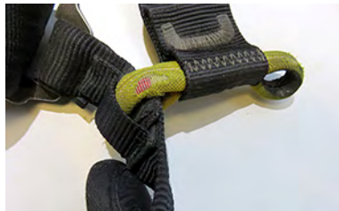
• Damaged attachment point
