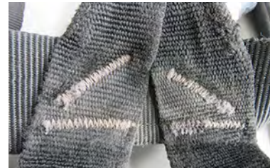
• Damaged safety stitching
