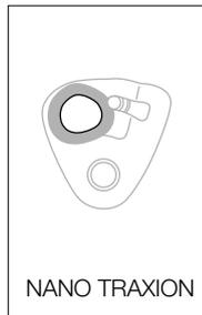
• Check the condition of the fixed side plate (marks, deformation, cracks, corrosion).
